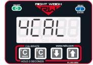
*\*In 4CAL mode, the scale can store four sets of calibration data for trailers that have various operating conditions.*
