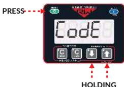
With the gauge off, press and hold both the C LOW and C HIGH buttons, then press the ON/OFF button. Release all three buttons. The gauge will display "Code".
