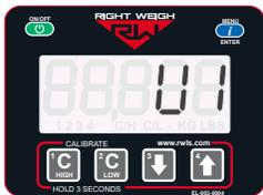
The gauge should be set to detect 1 Spring Sensor. See *Air/Spring Suspension Gauge manual* for more information on how to set the sensor configuration.
