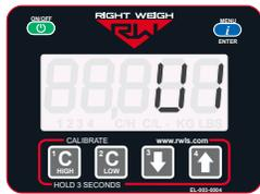
The gauge should be set to detect 1 Spring Sensor. See *Spring Suspension Gauge manual* for more information on how to set the sensor configuration.
