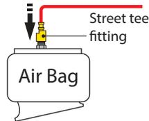
Insert new air line and fitting into the tee fitting
