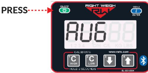
1: With the scale OFF, hold both the UP and DOWN arrow buttons, and press the ON/OFF button. Release all 3 buttons. The scale will display the current mode.
