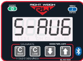
2: Press the UP arrow button to cycle through the configuration modes. To confirm your selection, turn the scale off by pressing the ON/OFF button.
