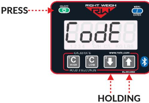
With the gauge off, hold both the C LOW and C HIGH buttons, then press the ON/OFF button and release all three.
