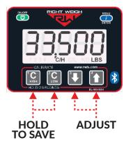
Use the UP and DOWN arrows to set the desired warning weight.
