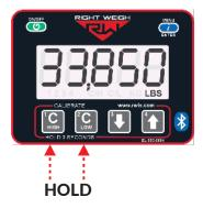
With the scale turned on, press and hold both the C HIGH and C LOW buttons until the "C/H" symbol appears.
