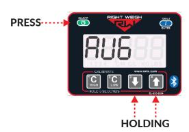
1: With the scale OFF, hold both the UP and DOWN arrow buttons, and press the ON/OFF button. Release all 3 buttons. The scale will display the current mode.
