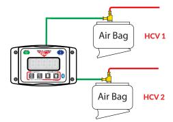
AIR UP SUSPENSION AND CHECK FOR LEAKS
