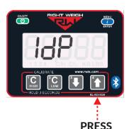
2: Press the UP arrow button to cycle through the configuration modes. To confirm your selection, turn the scale off by pressing the ON/OFF button.
