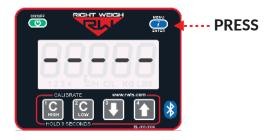
Press the MENU button and enter the new 5-digit PIN code using the 1, 2, 3, and 4 buttons. Press the MENU button again to save the code.
