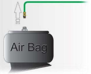
Insert the Street Tee fitting into the top of the air spring and then reattach the suspension airline into the Street Tee.
